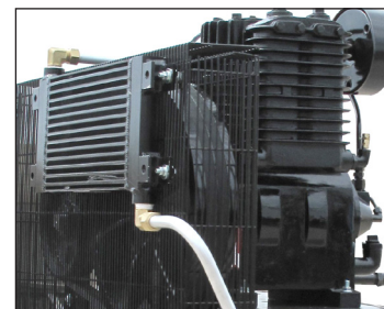
Air cooled after cooler Platinum unit
