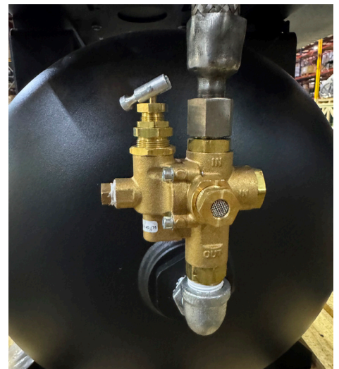
Pilot Valve for reed valve compressor pumps. This valve controls pressure and load/ unload running. (Do Not Adjust this valve, will void warranty if adjusted)
