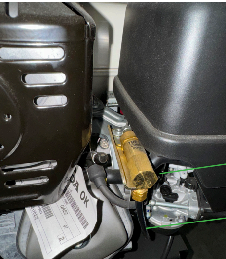
Throttle control Air signal for throttle control
